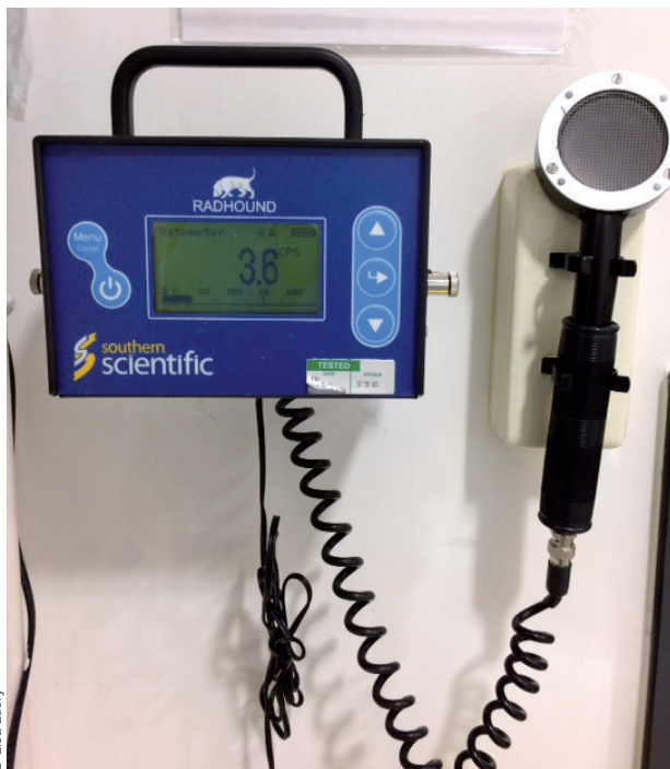
Figure 3. A Geiger counter can be utilized to ensure radioactivity levels are low enough to allow a cat to be discharged home; it also allows monitoring of hospital personnel.
