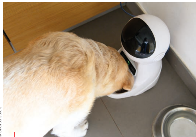
Figure 6. Electronic food hoppers which automatically measure out the correct daily portion can help with weight control, and some devices can also monitor food consumption throughout the day, allowing an owner to chart their pet's feeding pattern.
